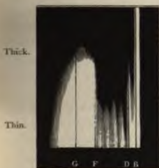
FIG. 79.—Absorption of various thicknesses of a solution of the salts of chromium. (Glaustone.)
